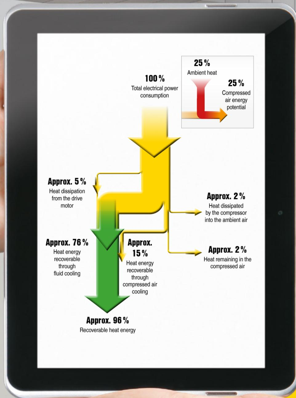
**Example savings calculation for hot air heat recovery for fuel oil (ASD 60)**
